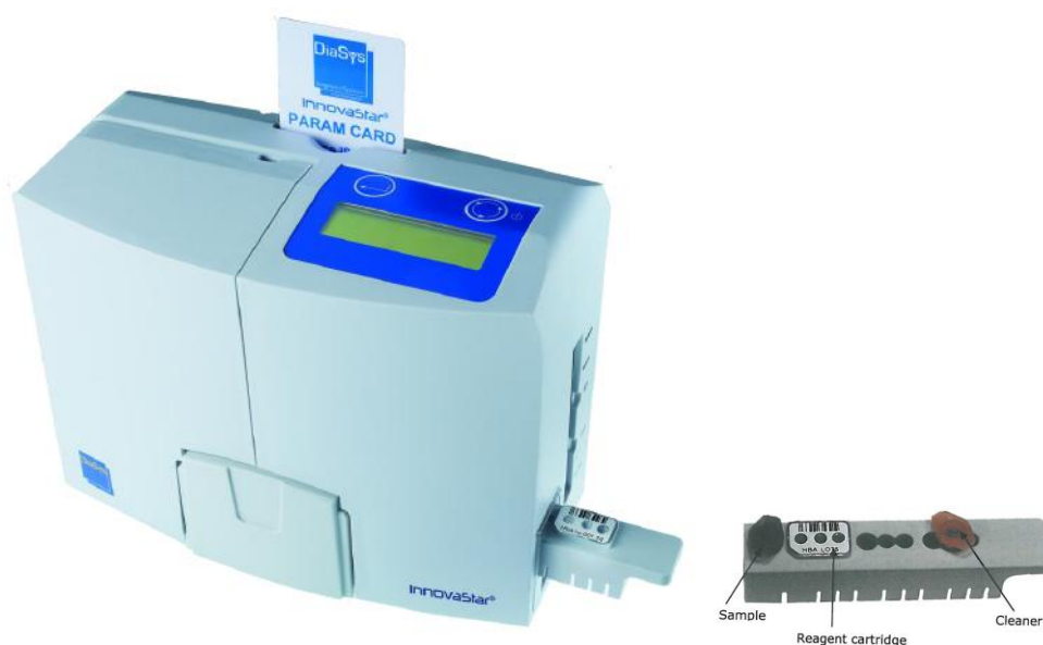
Figure 1a. The instrument InnovaStar including one HbA1c IS ParamCard (top).
