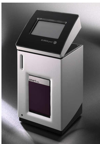
Figure 1. The Eurolyser smart laboratory photometer
